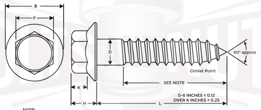
Minimum thread length is 1/2 length of the screw plus 0.50" or 6" whichever is shorter. Screws too short for the formula shall be threaded as close to the head as practicable.
