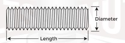
Material: ASTM A193/193M & ASME SA193/SA193M B7 Alloy Steel Threading: ASME B1.1 2A - Fully Threaded
