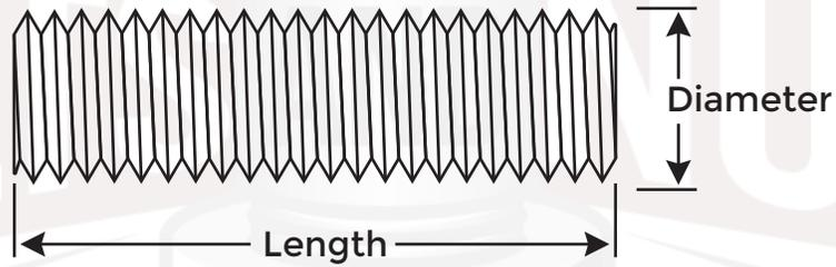
**Material: ASTM A193/193M & ASME SA193/SA193M B7 Alloy Steel**
